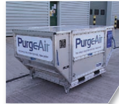
1. AKH Container PRG002AKH used where routine air transport is expected in A320 aircraft.
