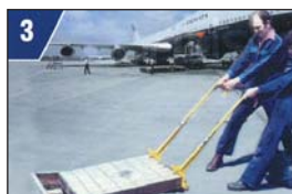
Slide back the cover on the EZI-LIFT rollers
