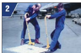
Gently pull back the EZI-LIFT's to raise one edge of the cover
