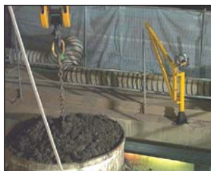
Angled Davit with 45m open-drum hoist
