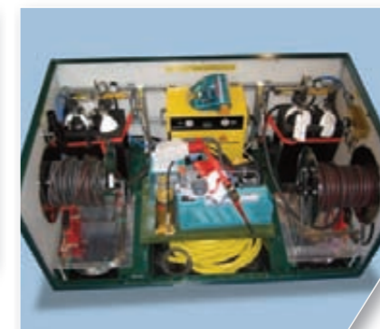
2. Flight Boxes – PRG002B used where routine air transport is expected in smaller aircraft down to Boeing 737's.
