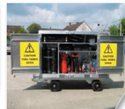
3. Modular Purge~Air PRG224 used as a hangar workstation, but can be transported by air. This modular system allows system components to be purchased separately.
