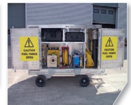
3. Modular Purge~Air PRG224 used as a hangar workstation, but can be transported by air. This modular system allows system components to be purchased separately.
