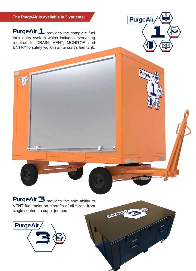
PurgeAir provides the ability to DRAIN, VENT and MONITOR fuel tanks on aircrafts of all sizes. It is also provided with suitably rated ancillary equipment to aid with any maintenance task within the tank.
