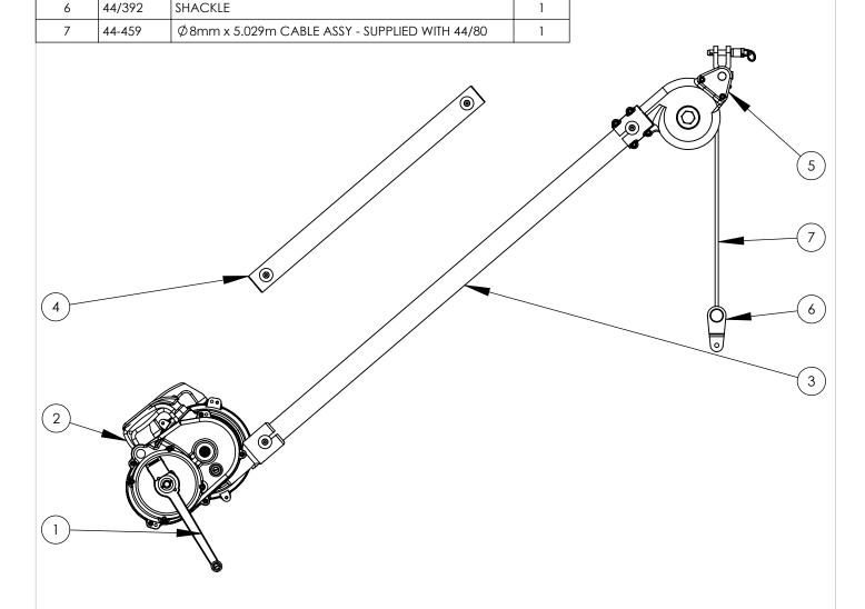
**HEIGHT OF LIFT:** 3.250m WHEN USING EXTENSION TUBE 44/90 3.770m WHEN USING EXTENSION TUBE 44/95
